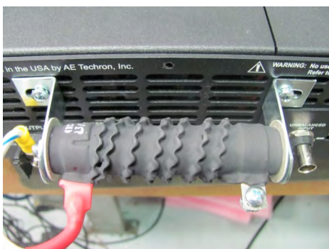
Figure 4.1 – 2105/7224 Ballast Resistor Mounting
