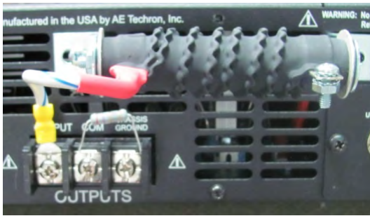
Figure 4.3 – 2105/7224 Ballast Resistor Connected to Output Terminal
