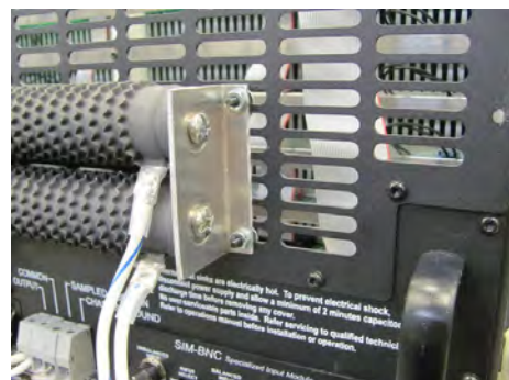
Figure 4.2 – 2120/7796 Ballast Resistor Mounting
