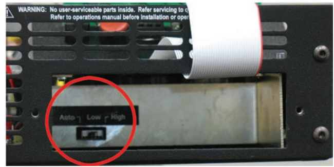
Figure 5.12 – Bi-Level Power Switch Location
