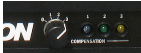
Figure 3.3 Amplifier Compensation Control
