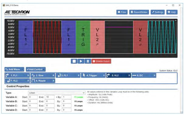
Now we need to assign Variable A to the Start Offset and Stop Offset properties in the DC wave segment. Click on this segment and you will notice that there is now a drop-down menu next to each property. Select "A" from this drop-down window for both the Start Offset and Stop Offset properties.
