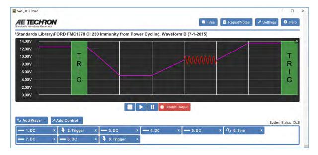
This is an actual test out of the Ford EMC standard. The segments and properties are set using the requirements established by Ford. Feel free to click around on the various segments to see how this test works.
