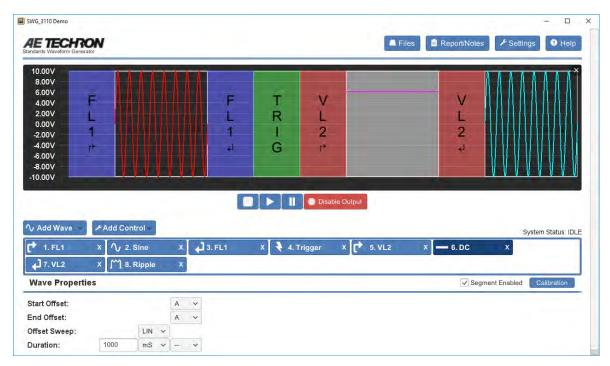
Now, when this test is run, the Start Offset and End Offset values of the DC segment will change each time this section is "looped." The first time through the loop, the values will be 0 volts, the second time the values will change to 1 volt, and so on until the values reach 11 volts. After that, the test will move on to the next segment in the test, in this example, the Ripple segment.
