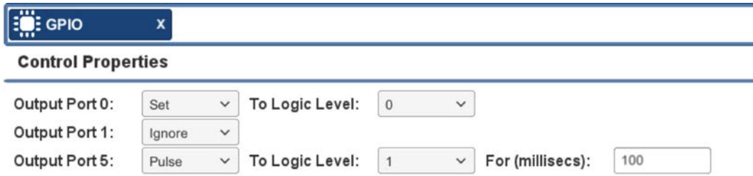
Figure 6.17 – GPIO Output Control Properties
